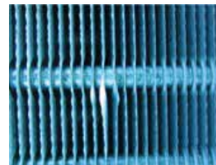
Cooling coil fins 60 day after UVC
